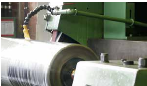
Grinding of pistons and cylinders between centers
