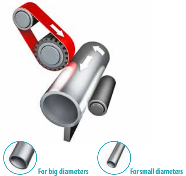
Centerless grinding of tubes and bars
