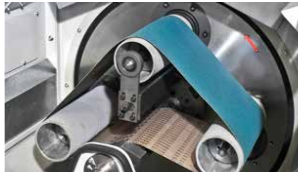
Descaling of coils using planetary grinding
