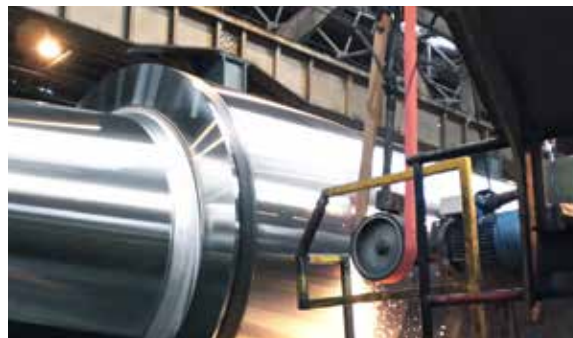
Cylindrical grinding of rollers on supporting rollers
