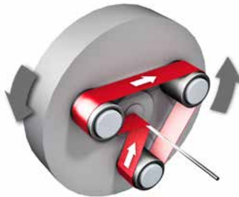
Descaling of coils using planetary grinding
