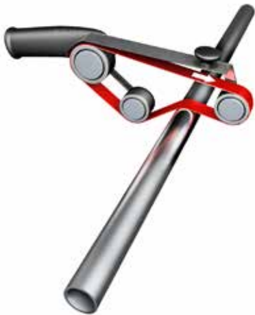
Cylindrical grinding of tubes and bars using power tools
