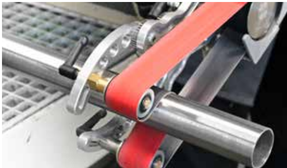
Cylindrical grinding of tubes and bars using power tools
